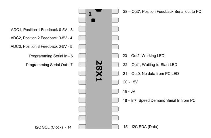
August 08 - IMPORTANT The PICAXE 28X1 chip programming has now been updated to allow newer 28X1 Firmware A.3 chips to be used. Make sure you are using the SPU\_I2C\_16.bas program and have an external 16MHz resonator fitted to the chip on the breadboard (pins 9 & 10) if you are using a A.3 firmware chip.
