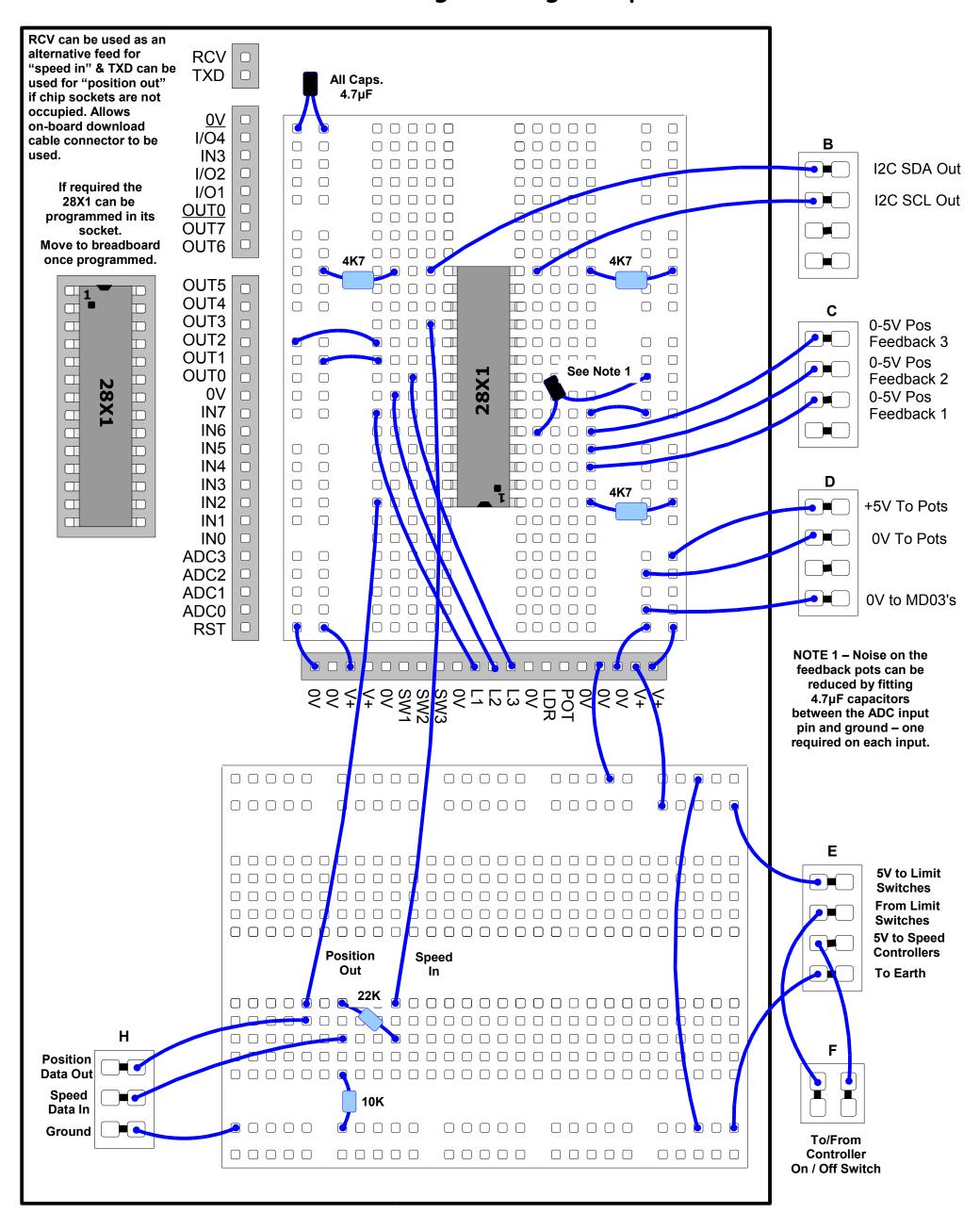
August 08 - IMPORTANT The PICAXE 28X1 chip programming has now been updated to allow newer 28X1 Firmware A.3 chips to be used. Make sure you are using the SPU\_I2C\_16.bas program and have an external 16MHz resonator fitted to the chip on the breadboard (pins 9 & 10) if you are using a A.3 firmware chip.
